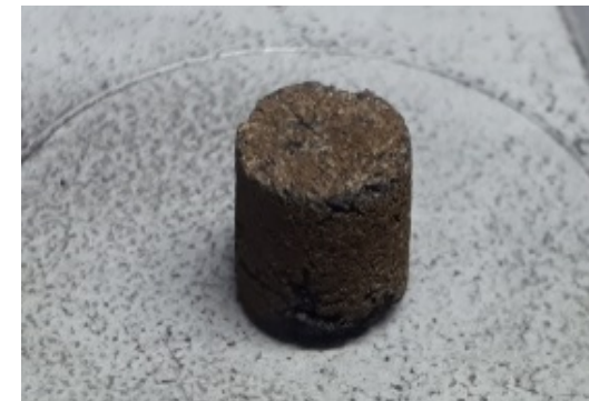
Simulated fuel debris for testing
